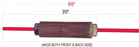
COTTON REEL HOLDER MADE OF WOOD BATTEN,PLY&UTE STRINGS WITH WEATHER COAT COLOURING OVER POP FINISH.
